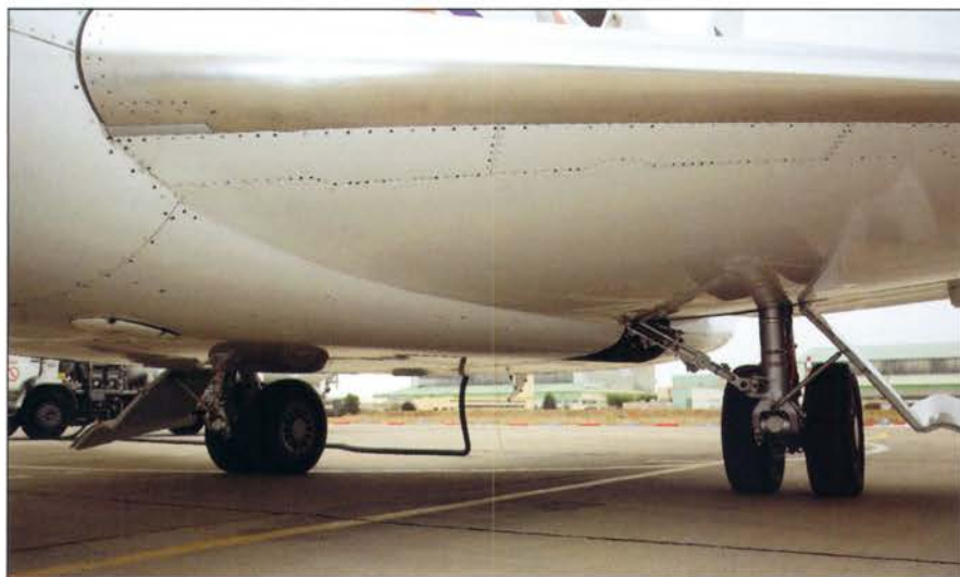
The 7X's wing is thicker at the root and thinner at the tip than the 1970's-vintage Falcons' airfoil.
