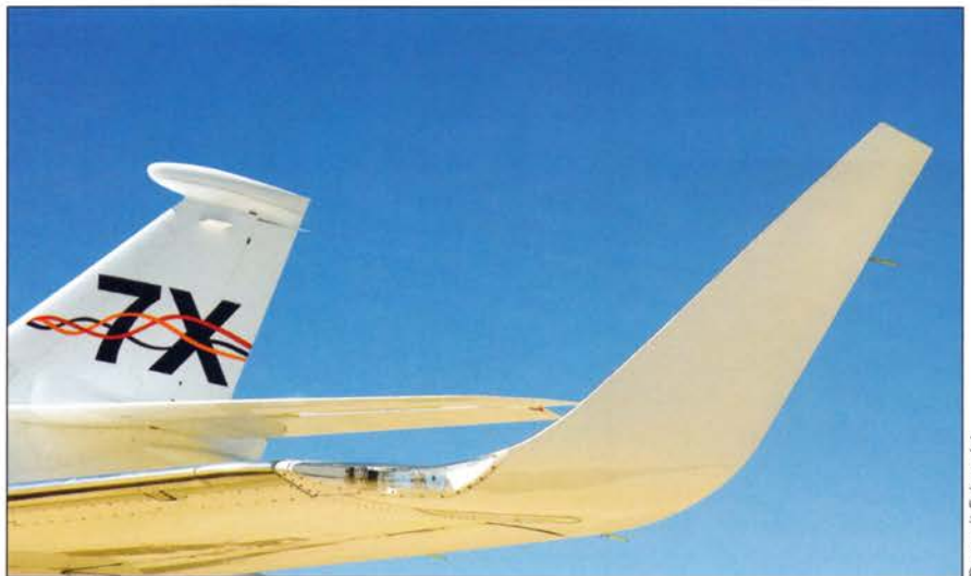
The decision to fit the 7X with winglets was made about six months into program development when Dassault elected to increase range from 5,700 nm to 5,950 nm.
